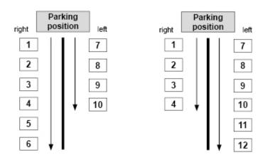
If the number of boxes differs between the left and right sides, the number of stopping positions on the side with more positions must be entered in the setup by a service technician (see illustration).
