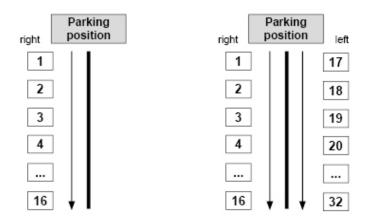
**Note:** After initial installation, a magnet is attached to the corresponding box. If the boxes are subsequently moved the magnets must also be adjusted. If a box is removed, its box number must be left out during registration. Note that one magnet serves two boxes facing opposite each other.
