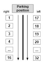
The automatic feeder starts counting at the right-hand box closest to the parking position. The corresponding numbers must be assigned depending on how many calves are registered and to which box (see 4.1 "Manual registration of animals" - 23).
