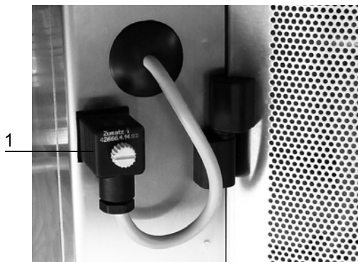
1 Device socket on machine housing
