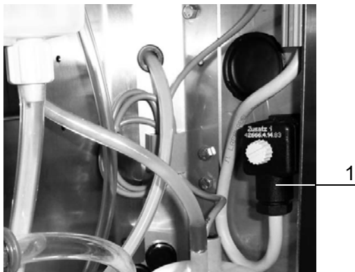
1 Device socket in the machine housing
