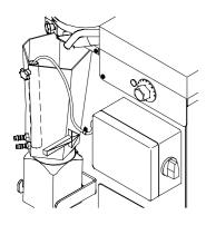
Always lay the cable between the pressure tube and the pressure switch towards the bottom. In case the milk flows into the pressure tube, the latter will become inoperative.
