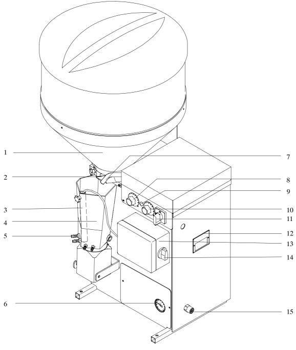
1 = Milk powder hopper 9 = Pilot lamp for heating2 = Dosing slide10 = Heating thermostat 3 = Pressure tube11 = Main switch ON/OFF (not for **TAP0-EZ1-27**) 4 = Mixer12 = Rating plate 5 = Suction hose connection 13 = Power unit6 = Manometer14 = Program switch 7 = Milk/Water outlet 15 =Water supply 8 = Thermostat für minimum operating temperature (**not for TAP0-EZ1-27**)
