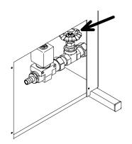
When the dispensed milk powder amount is too low, close the water control valve a little bit.
