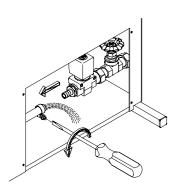
Drain the whole water from the boiler and the pressure reducer.
