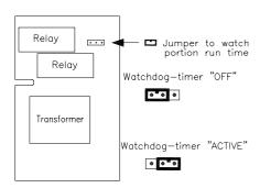
The pressure switch connected to the pressure tube switches the waterand powder conveyance off, as soon as a certain pressure has been reached. After several seconds a relay switches the mixer off. A portion is prepared as soon as the mixer is empty. In case of water deficiency the automatic feeder switches off automatically after approx. 40 seconds, provided that the jumper is in position ON.
