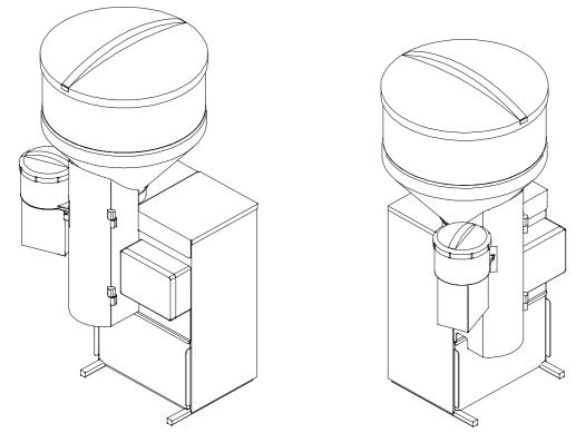
Drawing: Automatic Feeders with New Fly Protection and Dispenser for Powder Additives
