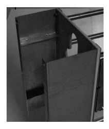
Screw the pipe ends (1) of the side panels.
