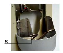
7. Finally screw on the flipping teat bracket with both angle brackets.
