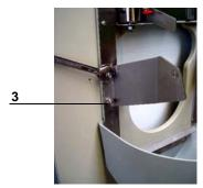
3. Unscrew the lower splash guard (4) to which- among others - the dribble bowl (5) is secured, with a Phillips screwdriver.
