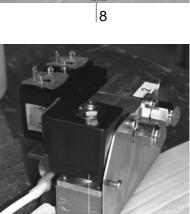
Insert the valve unit and connect the female connectors to the male connectors of the valves.
