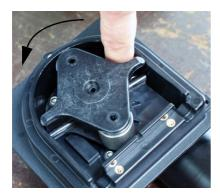
**ATTENTION** Use only the supplied silicone grease. Another silicone grease can damage the pump housing and the pump hose.
