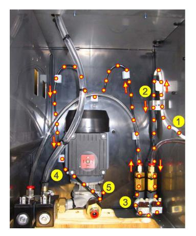
1. Feed the frost protection cable along the inside of the automatic feeder to the holder (1).
