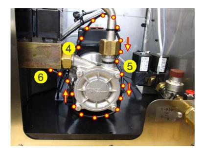
5. Fix the frost protection cable on the milk pump (5) and feed it to the flush valve (6).
