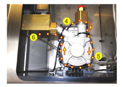
5. Fix the frost protection cable on the milk pump (5) and feed it to the flush valve (6).
