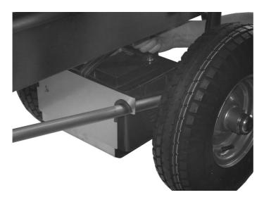
14. Screw the battery box and the suspended plate together by means of the supplied screw.
