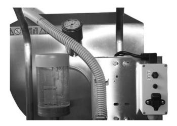
9. Run the cable of the dosing pump along the chassis of the MilchMobil towards the rechargeable battery and secure it with the supplied cable clips (see illustration).
