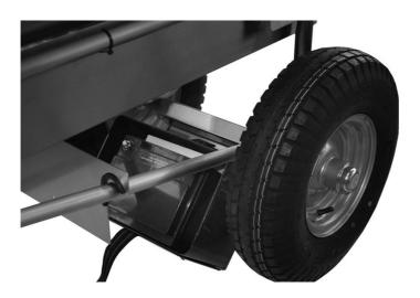
13.Pull the battery box upward by means of the lashing strap until it hangs horizontally in the chassis of the MilchMobil (see illustration).
