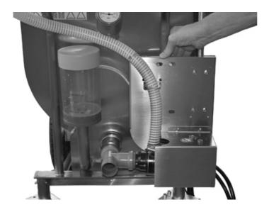
5. Tighten the U-bolts with the supplied washers and nuts evenly.
