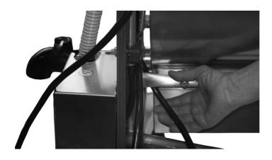
9. Run the cable of the dosing pump with portion control along the chassis of the MilchMobil towards the rechargeable battery and secure it with the supplied cable clips (see illustration).
