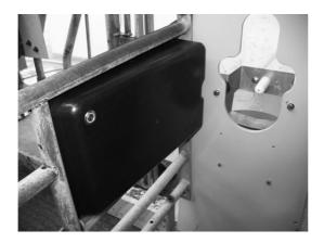
4. Feed the antenna cable through the cable opening that you drilled before.
