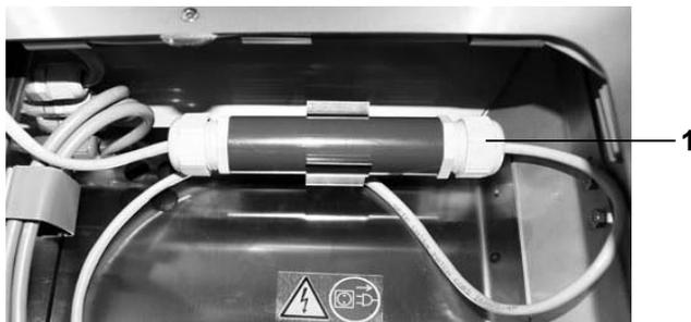
1 Cylinder with Ethernet connection
