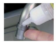
22.Cut the detergent hose diagonally so that residual detergent can be removed by the water jet at the end of the cleaning cycle.
