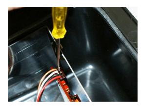
4. Open the securing nut of the push button
