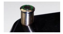
6. Make sure the O-ring is placed between the button and the housing and insert the button into the hole of the housing.
