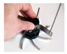
9. Install the new spring star in the powder hopper.
