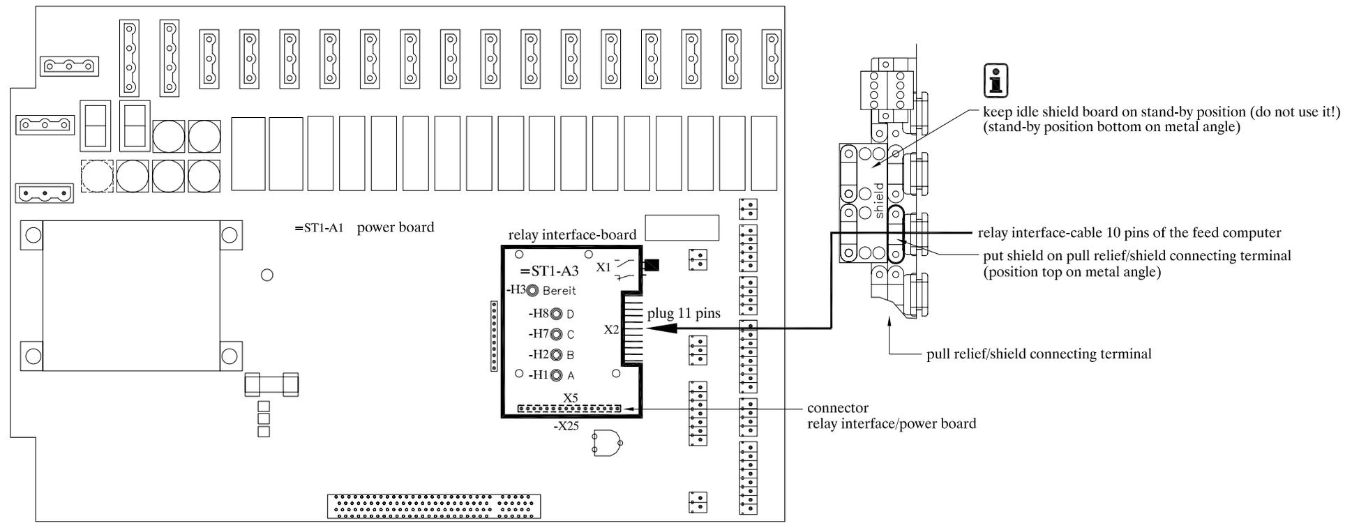
also see the wiring diagram of the machine
